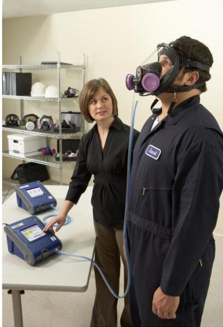
Widely used particle counting face-fit testing equipment
